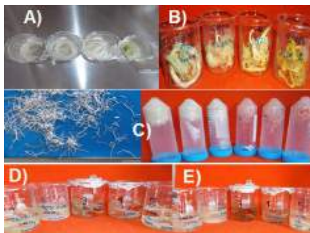
Figure 3. Chemistry and physical tests in the fiber (Agave salmiana). A) y B) Fiber before and after attack at different concentrations of NaOH, C) Appearance and granulometry (0.42-1.42mm) of the fiber employed in the determinations. Test to determine the water retention capacity and retention capacity of organic substances (edible oil), D) Fiber before and E) After to attack by salt (NaCl) and acid (HCl) at differents concentrations.
